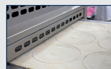
4. Product cutting: cutting products out of the dough sheets. Multiple shapes and sizes are possible.
