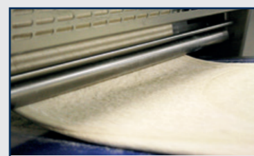
2. Reduction stations: reduces the dough sheets thickness to the final thickness.
