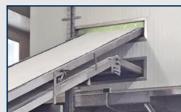
3. Proofing: enables the dough to develop its structure and helps to develop taste.
