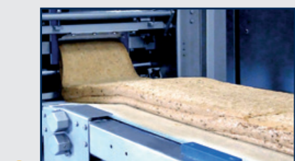
1. Pre sheeters: generate a homogeneous and stress-free dough sheets of any type with excellent weight control at the highest quality. The dough structure is untouched.
