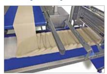
The belt with the dough sheet moves back and forth above the next conveying belt, this is an asymmetric lamination system. Suitable for soft dough and no restrictions regarding laminating width.
