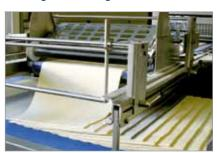
A guillotine cuts the dough sheet into regular rectangular sheets which are then stacked on top of each other. This flexible symmetric system lays even and uneven layers. Suitable for soft doughs and no restrictions regarding laminating width.
