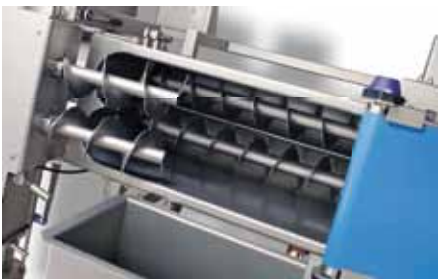
Automatic feeding section to feed the fat blocks into the fat pump hopper.
